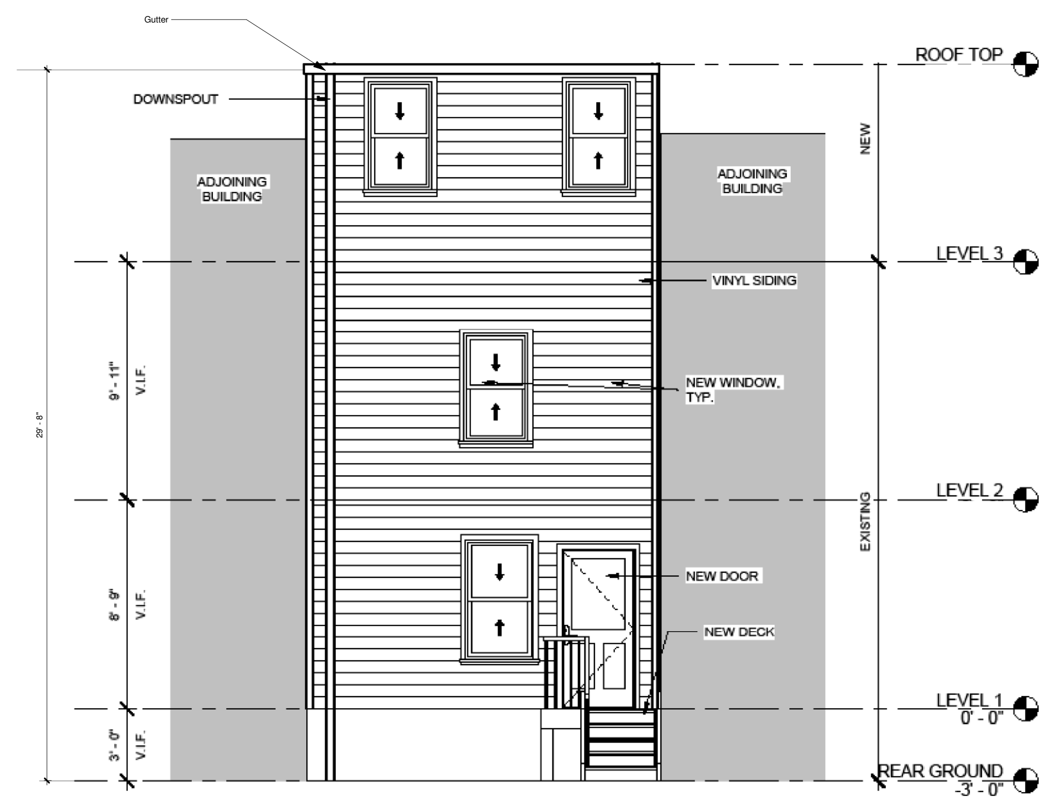
② SOUTH ELEVATION 1/4" = 1'-0"
