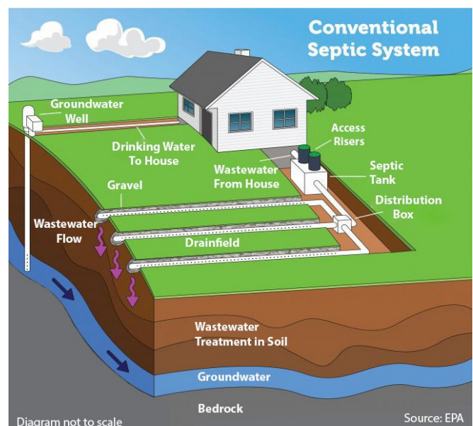
Figure 1. Diagram of a conventional septic system with a tank and soil dispersal area or drainfield.
