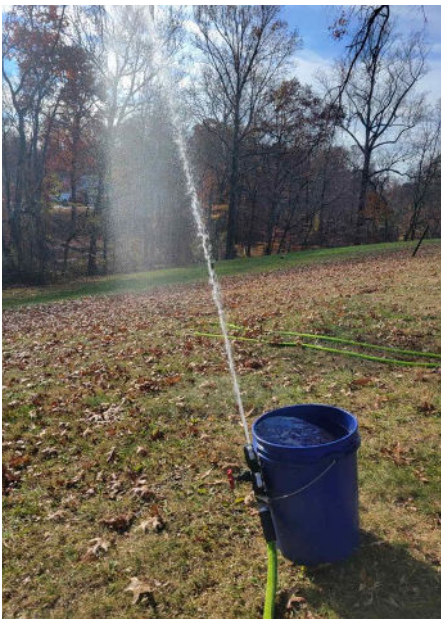
Bucket and gauges used to monitor pressure and flow
