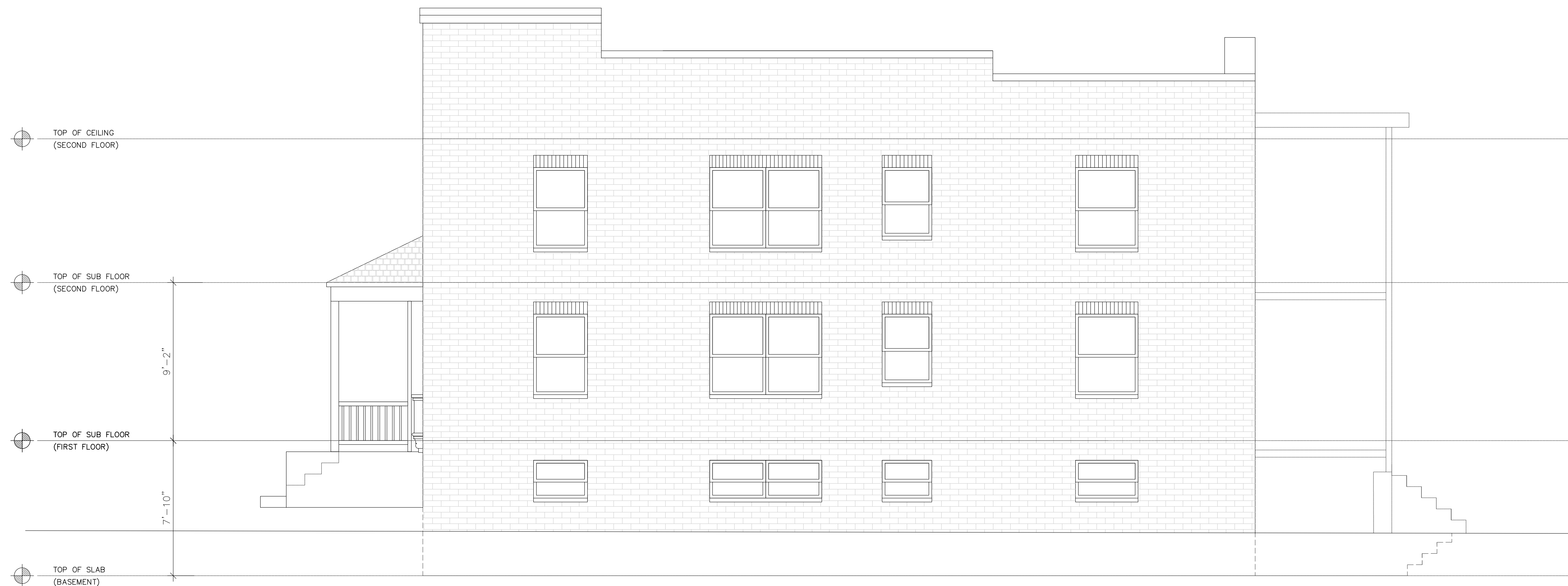
EXISTING RIGHT ELEVATION SCALE: 1/4" = 1'-0"
